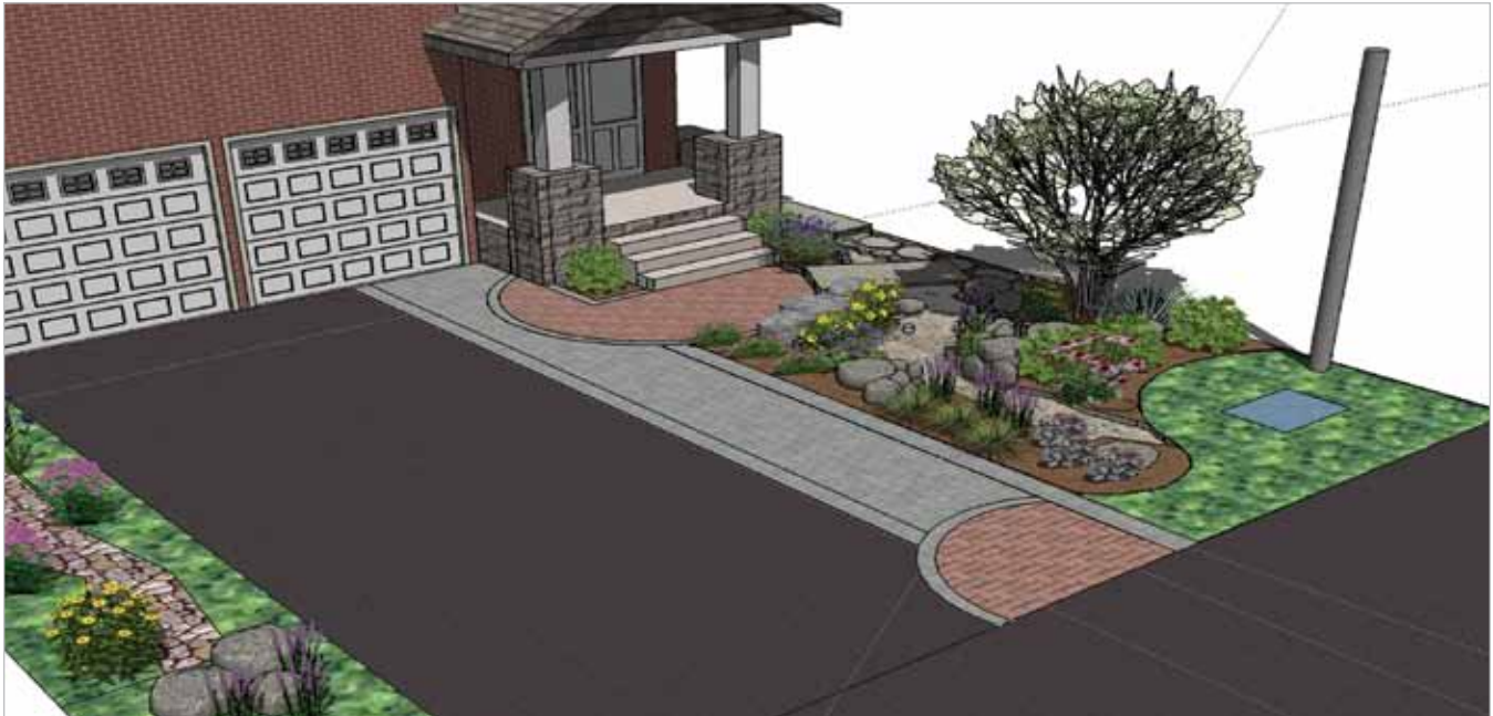
One of two Front Yard Makeovers – an eco-landscaping design for busy commuters featuring soakaways, a rain garden, a high-capacity rain barrel, permeable paving, and native and water efficient plants.
